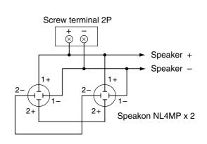
• Two speaker systems can be operated in parallel by connecting them in a cascade configuration as shown at right.
